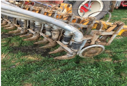
FIGURE 8 A) DIGESTATE INJECTION SYSTEMS: OPEN SLOT SHALLOW INJECTION ON THE LEFT; B) CLOSED SLOT SHALLOW INJECTION ON THE RIGHT (SOURCE: CIB – CONSORZIO ITALIANO BIOGAS)
