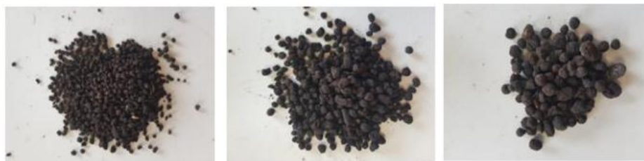
FIGURE 16 DIGESTATE-BASED GRANULATES OF DIFFERENT SIZES (SOURCE: ALGAE LLDC)
