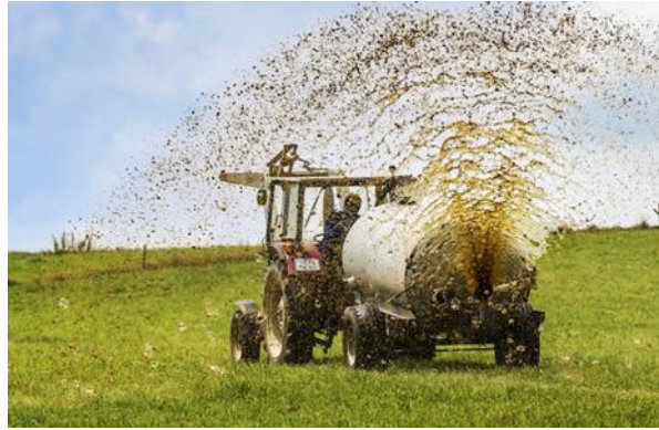
FIGURE 4 CONVENTIONAL DIGESTATE DISTRIBUTION EQUIPMENT (SOURCE: CIB – CONSORZIO ITALIANO BIOGAS)
