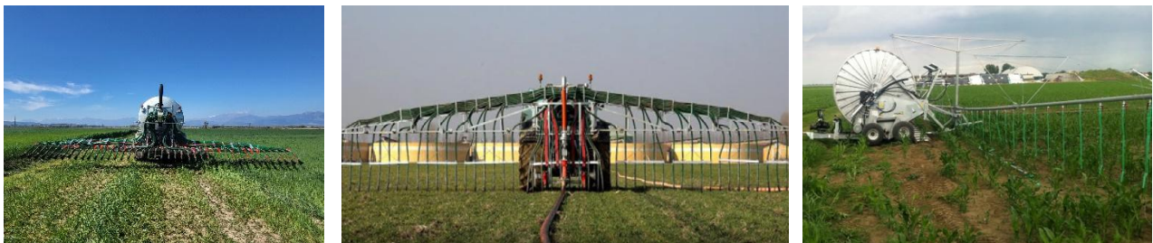
FIGURE 5 LOW-PRESSURE GROUND LEVEL DIGESTATE DISTRIBUTION (SOURCE: CIB – CONSORZIO ITALIANO BIOGAS)
