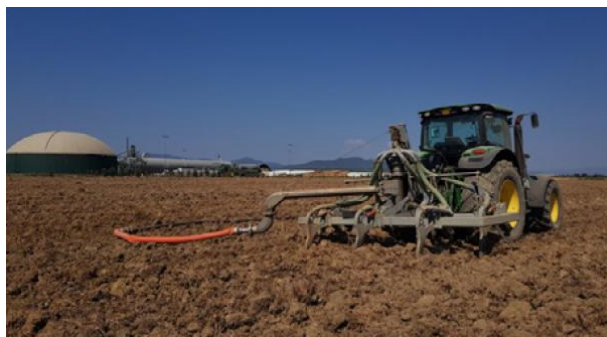
FIGURE 7 UMBILICAL DISTRIBUTION SYSTEMS. MINIMUM TILLAGE INJECTOR (SOURCE: CIB – CONSORZIO ITALIANO BIOGAS)
