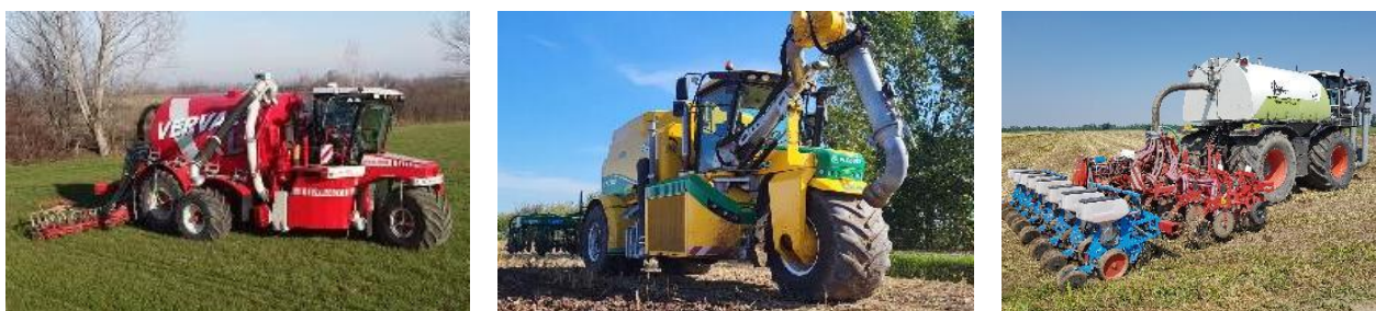
FIGURE 11 INNOVATIVE TANKER TRUCKS FOR LOW-PRESSURE SURFACE APPLICATION AND INJECTION APPLICATION OF DIGESTATE (CIB)
