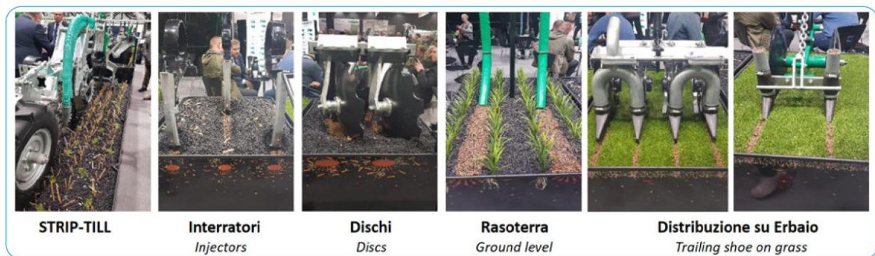
FIGURE 9 DIFFERENT TYPES OF ELEMENTS FOR DIGESTATE DISTRIBUTION (SOURCE: CIB – CONSORZIO ITALIANO BIOGAS)
