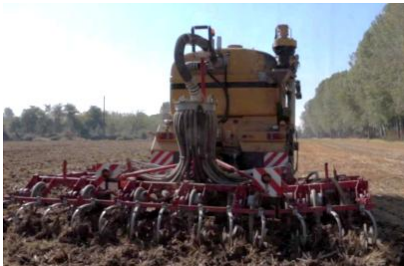
FIGURE 19 EXAMPLE OF ACQUA E SOLE EQUIPMENT FOR INJECTION OF DIGESTATE IN SOIL AT PRE-SOWING (SOURCE: SYSTEMIC PROJECT, 2017)
